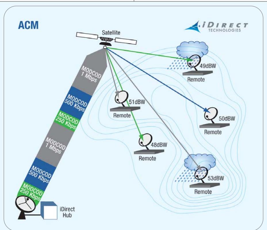
**Figure 1.** ACM enables each remote to achieve maximum data throughput by utilizing the most efficient coding and modulation scheme dependant upon the location within the satellite contour, antenna size, and clear sky conditions versus rain fade.
